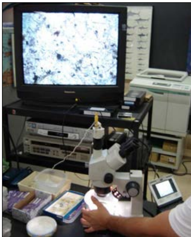
Photograph 4. Microfauna analysis using a trinocular video microscopy system.
