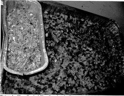
Picture 4 – Clean Crushed Glass Sample After Removal of Deleterious Material. Deleterious Material (Left).
