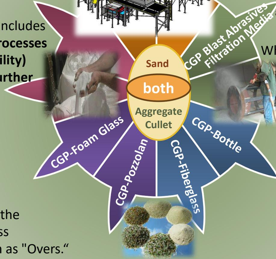
The output of our CGP is ready to be shipped to a bottle, fiberglass, foam glass, or pozzolan manufacturer. Or it can be used for glass blast abrasives and filtration media.
