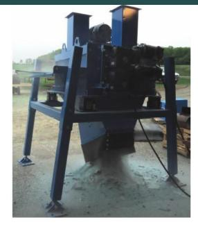
The Andela Windshield Stripper is simple to operate and maintain. A great machine for separating glass from laminate while reducing the glass into an aggregate.
