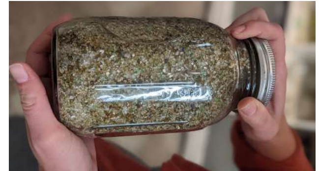
Waste glass is reclaimed & crushed to use as a sand substitute in GSI soils.
