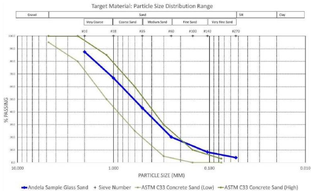
Figure 3: Particle size distribution of target glass-sand compared to ASTM C-33 concrete sand.
