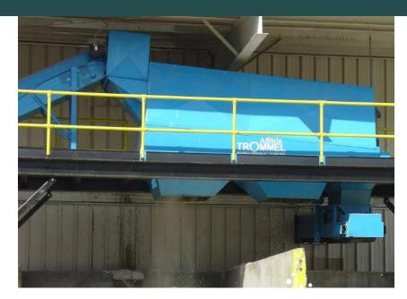
The Andela Trommel Screen Separator is designed to separate and size aggregate using woven wire mesh or perforated plate.
