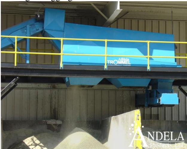
7. The non-glass will exit the end of the trommel screen and may go to an Eddy Current Separator for recovery of aluminum.
