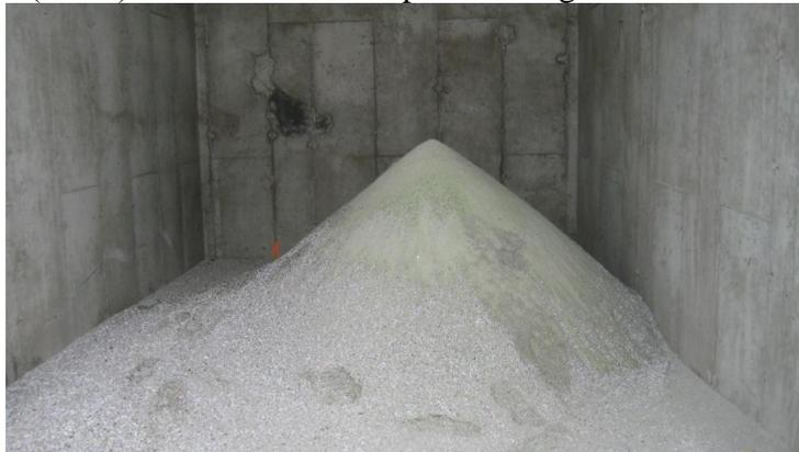
5. The second section has a larger screen (7/16") to remove the gravel sized glass. The glass may be mixed with paper shred and small plastic bits. The paper removal system uses a blower to remove the paper shred as the material falls out of the trommel screen. The glass gravel may fall into a bunker or be transferred by conveyor back into the pulverizer for re-grind into glass sand.
