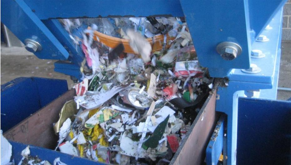
2. The mix is transferred by conveyor into the Andela Pulverizer. It may go under a cross-belt magnet to remove metal.
