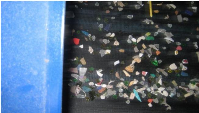
6. The pulverized glass does not have any sharp edges. The gradation of the pulverized sand and gravel will meet engineered aggregate specifications. The pulverized glass aggregate will have 1% or less organic content. The system will reduce 95% of the glass into a 7/16" minus glass aggregate.
